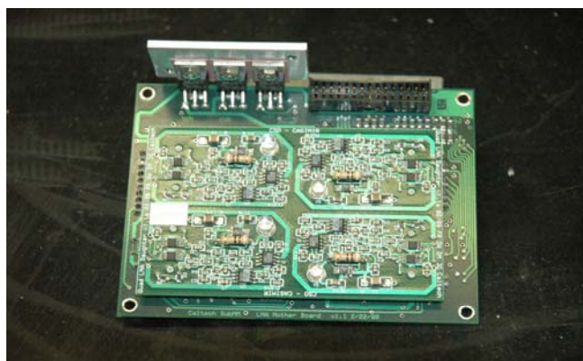
Fig. 5. Receiver bias electronics developed in collaboration with CSO. These circuit boards are for biasing the low-noise amplifier (LNA) on the cold LHe work surface of the receivers. These electronics are fully automated and controlled via computer interface, and also have the capability for manual control, allowing them to be used during mixer development
