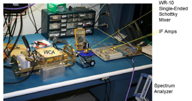
Fig. 12 Photograph of prototype AM noise test set.
