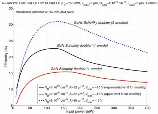
Fig. 9 Performance comparison between a 200 GHz GaAs Schottky doubler (featuring 8 anodes with a 350 nm epilayer) and a 200 GHz GaN Schottky doubler (featuring 1 anode with a 650 nm epilayer).
