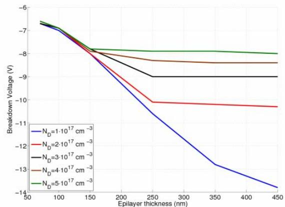
Fig. 37 DC breakdown voltage as a function of the epilayer length and doping for GaAs Schottky diodes.
