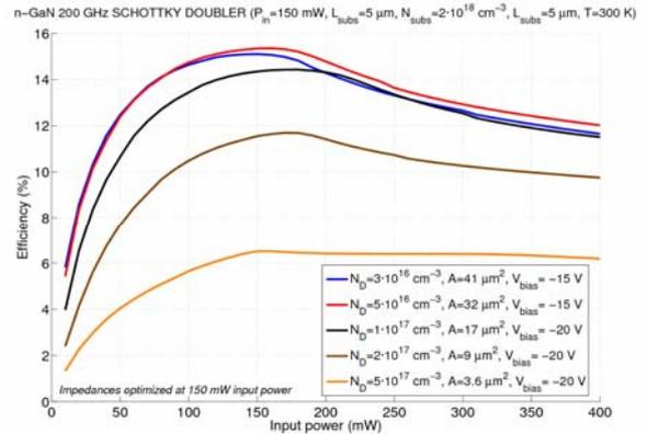
Fig. 40 Simulated performance of a 200 GHz GaN Schottky doubler as a function of the input power and the epilayer doping level. Bias and anode areas have been optimized for a 150 mW input power.
