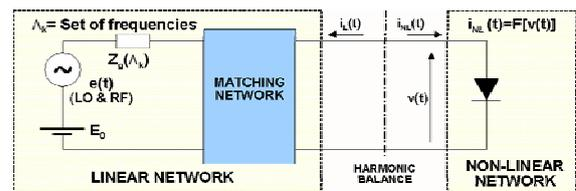
Fig. 34 General scheme of the numerical Harmonic Balance simulator for the design and optimization of Schottky- diode-based circuits at millimeter and submillimeter-wave bands.
