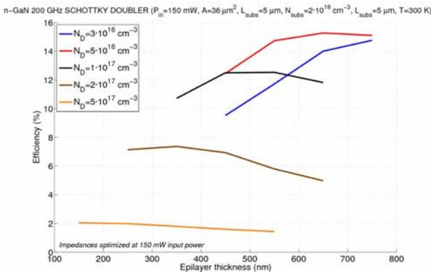
Fig. 39 Simulated performance of a 200 GHz GaN Schottky doubler as a function of the epilayer thickness and the doping level (anode area is  $36 \mu\text{m}^2$ ).
