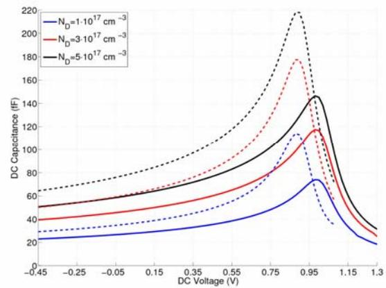
Fig. 36 DC capacitance curves for GaAs (dashed lines) and GaN (solid lines) as a function of the epilayer doping.
