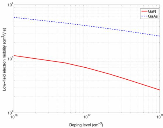
Fig. 35 Low-field electron mobility for GaAs and GaN as a function of the epilayer doping.
