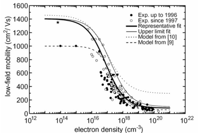
Fig. 41 Measured low-field mobility for wurtzite n-GaN as a function of doping density (reprinted from [1]).
