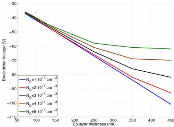
Fig. 38 DC breakdown voltage as a function of the epilayer length and doping for GaN Schottky diodes.
