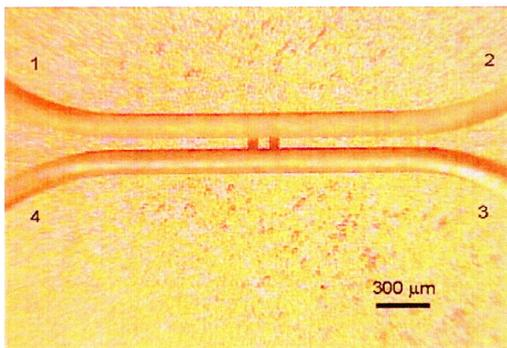
Fig. 1 A photograph of a 10-dB directional coupler at the Band 10 frequencies.
