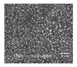
Fig. 1. SEM micrograph of ZnSe nano-dots.
