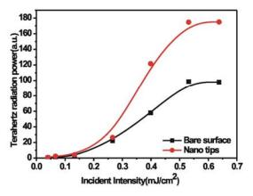
Fig. 2. THz fluence as a function of pump fluence for nano-dot and bulk ZnSe samples.
