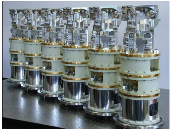
Fig. 3. Six Band 9 pre-production cartridges (#3-8) assembled, tested, and awaiting acceptance and delivery to the ALMA project in Aug. 2007.
