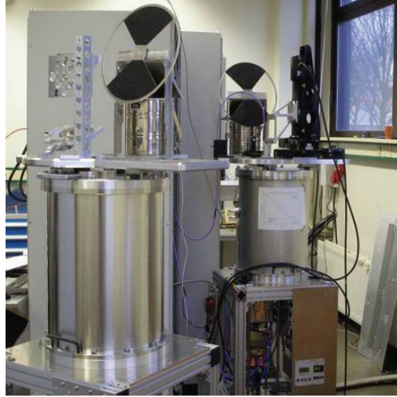
Fig. 4. Two cartridge test cryostats (from NAOJ, Japan). With a test throughput of 1 cartridge per 3 weeks, a 2 nd test system was built in 2007-2008 to allow a delivery rate of 2 cartridges per month to be realized.
