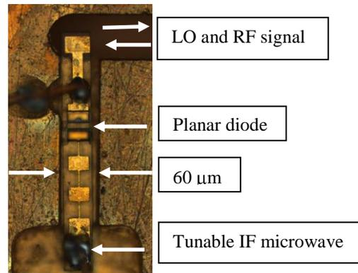
Fig. 5. Photograph of 1.6 THz integrated SBG circuit mounted in an open metal block. The circuit channel width is  $60 \mu\text{m}$ . The varactor is pumped by a tunable IF microwave signal. The output RF signal will be LO  $\pm$  IF.
