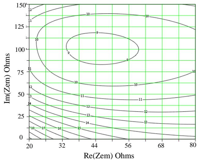
Fig. 4. ADS Simulated conversion loss corresponding to different embedding impedances for  $1 \mu\text{m}$  diameter anode.
