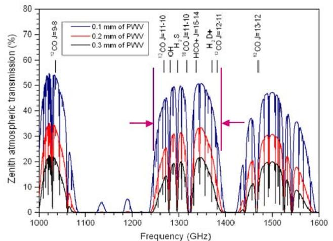
Fig. 2. Atmospheric transmission on the Llano Chajnantor for different weather conditions from 0.1 to 0.3 mm PWV. 0.3 mm is already considered excellent condition for observations until ~900 GHz, but is insufficient for the 1.3 THz window.
