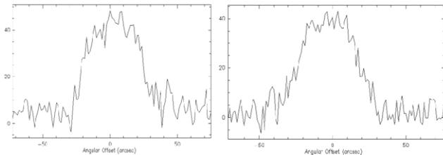
Fig. 15. Jupiter pointing in elevation (left) and azimuth (right).
