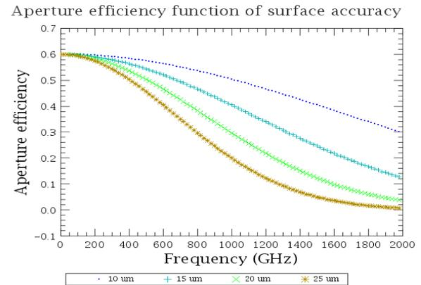
Fig. 14. Aperture efficiency dependency on surface accuracy. Best achievable results seem to be about  $15 \mu\text{m}$  rms after a panel adjustment session but  $20 \mu\text{m}$  rms is more likely to be the average value after few months.
