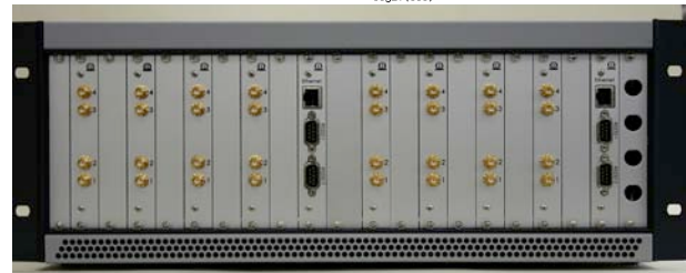
Figure 7: Measured Allan variance of the Supercam spectrometer system, including the Caltech IF processor. Allen time is 650s (top). The Supercam spectrometer system, built by Omnisys AB (bottom). This single 3U crate can process 16 GHz of IF bandwidth at 250 kHz spatial resolution. It consumes less than 200W of AC power.
