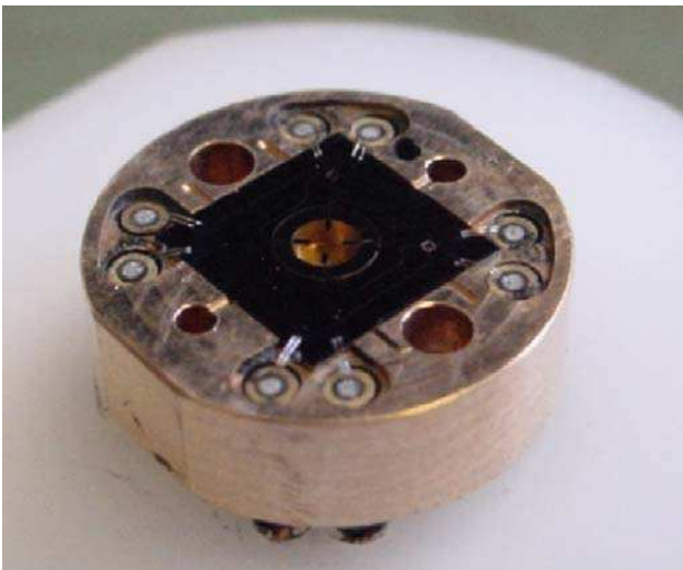
Figure 15. A prototype HF detector mounted in the detector module block. Bias signals and heater power are taken from the two TES detectors on superconducting pins through the block to the readout system on the back of the focal plane array. The circular waveguide back-short is visible through the centre of the detector chip.
