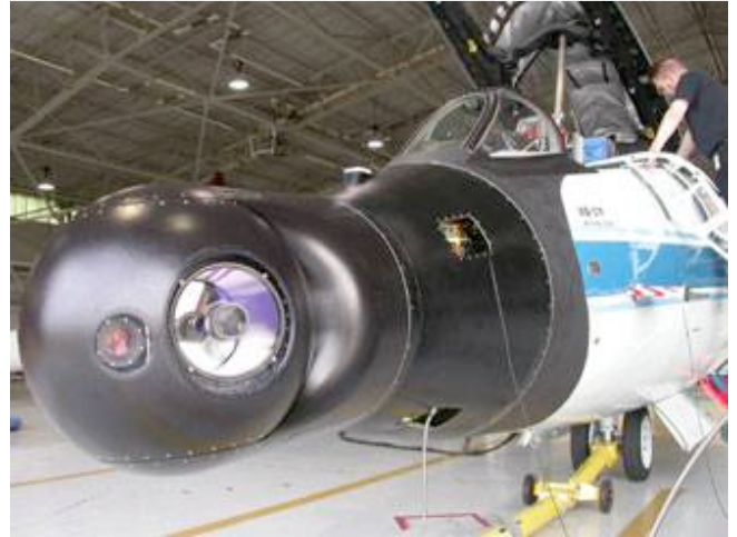
Figure 8: The WAVE system mounted on the nose of a WB-57F. ATOMMS will replace the optical telescope in this system. A microwave transparent radome will replace the front skin and optical window.
