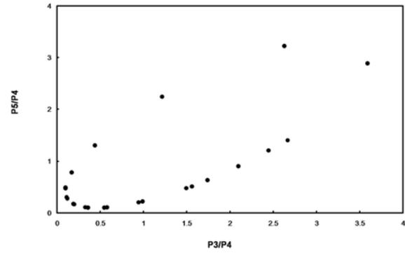
Fig.6. Ellipse curve from the first step calibration for WR15 six-port reflectometer at 61 GHz as an example.
