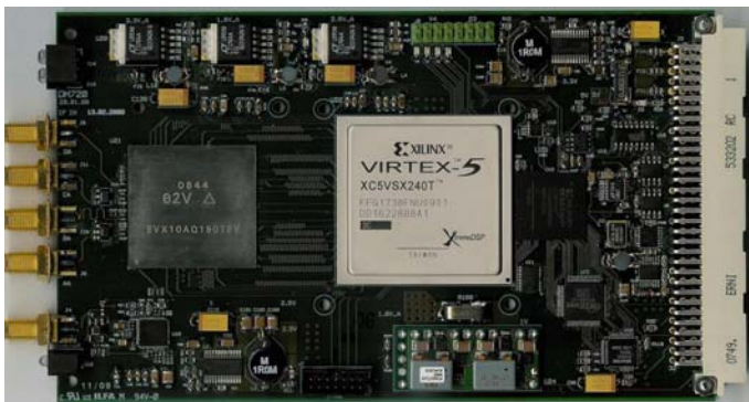
Fig. 3. Currently in lab tests: The new 2.5 GHz bandwidth XFFTS, making use of a first sample of E2V's 5 GS/s 10-bit ADC and the high performance Xilinx Virtex-5 SX240T FPGA.
