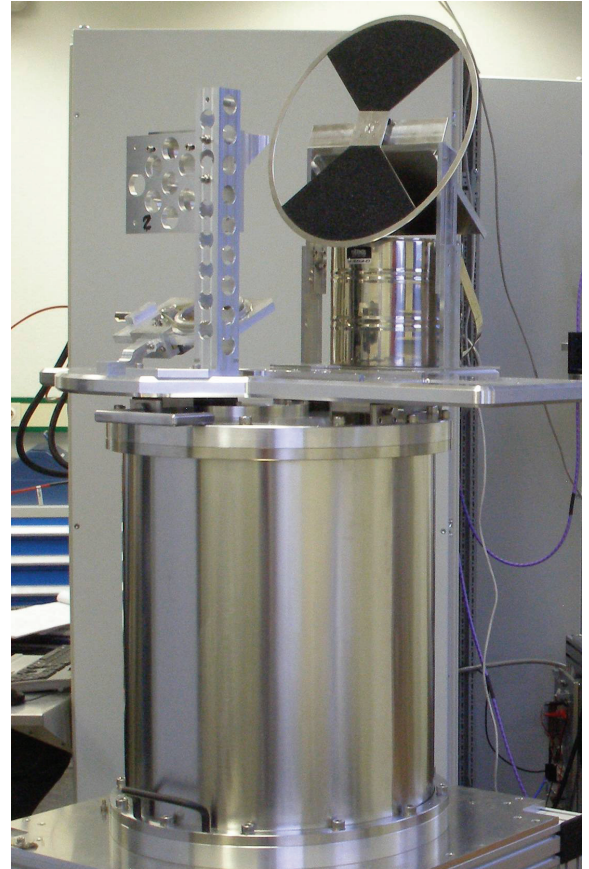
Fig. 2 – The Band 9 cartridge test system configured for polarization efficiency measurements, with a rotating polarizing grid placed between the receiver and the hot-cold load (both computer-controlled).
