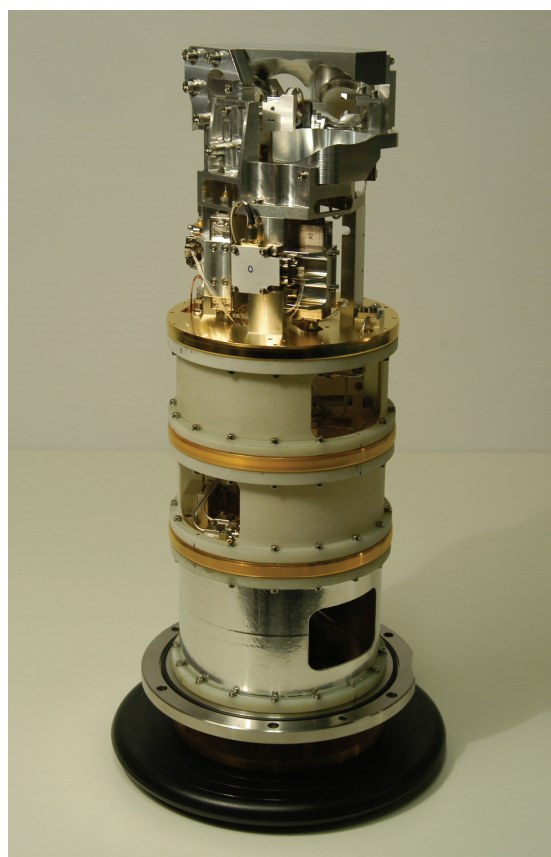
Fig. 1 – An ALMA Band 9 cold cartridge (i.e. not including the cartridge's warm electronics units). The cartridge is roughly 50 cm tall and 20 cm in diameter.
