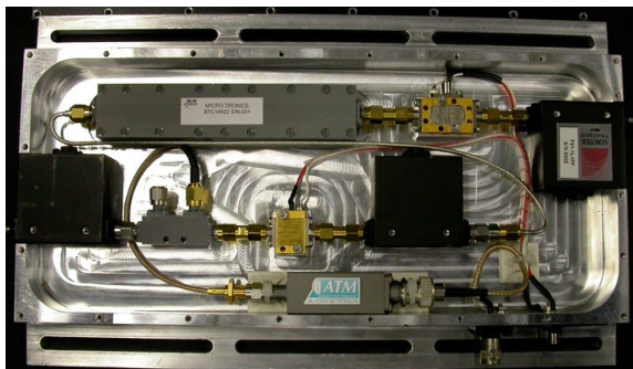
Fig. 4. 2-4 GHz IF chain with internal noise diode described in [7].
