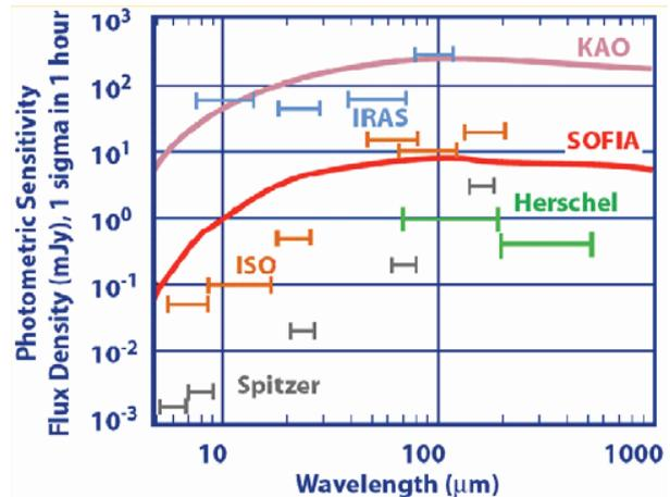
Fig.6. SOFIA's photometric sensitivity will be comparable to that of ISO.
