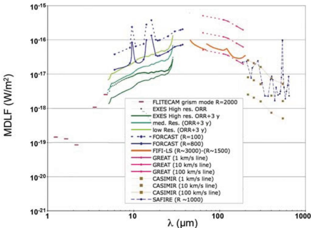
Fig. 8 (Above) The expected line sensitivity of SOFIA spectrometers at the time of full operational capability. Shown is the  $10\sigma$  minimum detectable line flux (MDLF) in watts per meter squared for 900 seconds of integration on source. Observing and chopper efficiency have not been included.
