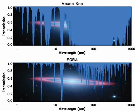
Fig. 2. The typical atmospheric transmission at an altitude of 45,000 feet as compared to the transmission on a good night at Mauna Kea (13,800 ft. MSL). From 1 to 1000  $\mu\text{m}$ , the average transmission is  $\geq 80\%$  except in the center of absorption lines due to mostly  $\text{H}_2\text{O}$ ,  $\text{CO}_2$ , and  $\text{O}_2$ . Background image: IRAC false color image of the Sombrero Galaxy, courtesy of NASA/JPL-Caltech.
