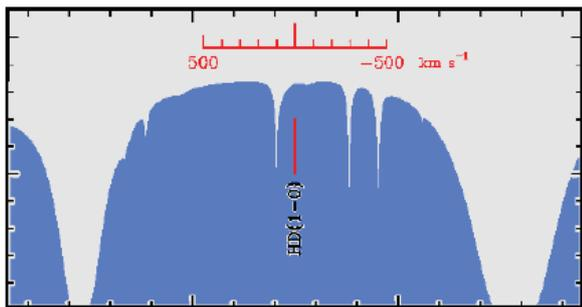
Fig. 12. Schematic representation of the atmospheric transmission around the 2.6 THz (112 μm) HD line at 40,000 feet
