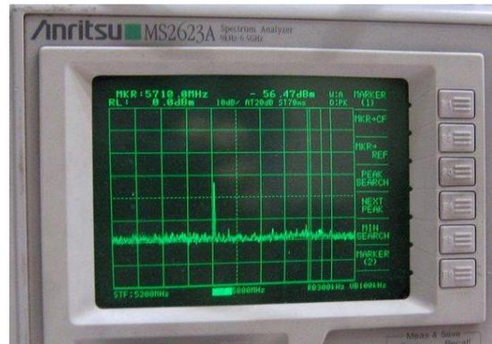
**Figure 4:** (Left) End-to-end testing of the entire STO instrument using the ambient temperature Schottky receiver and a 330 GHz test transmitter placed ~50m away from the telescope. (Right) Spectrum analyzer view of the Schottky receiver IF, showing the test transmitter tone passing through all telescope and instrument optics and downconverted and amplified by the IF processor. This test represented the final “go” for launch.
