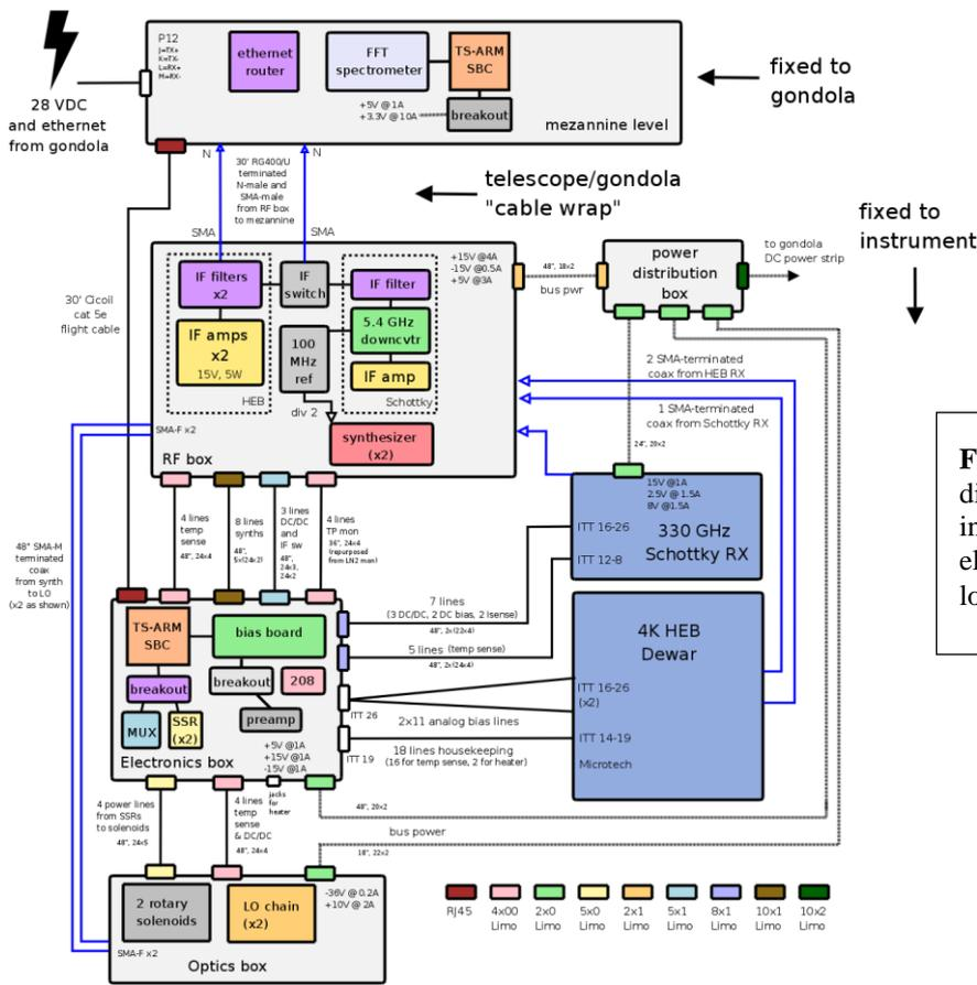
**Figure 3:** Detailed block diagram of the instrument control electronics and their location on the gondola.
