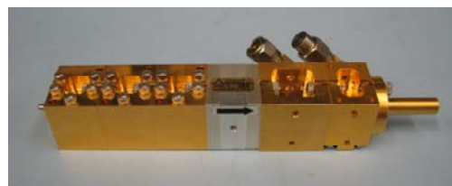
Fig.1: Schematic block diagram and photo of the 900 GHz LO chain, including power amplifiers, an isolator, two stages of frequency triplers, and a corrugated output horn.
