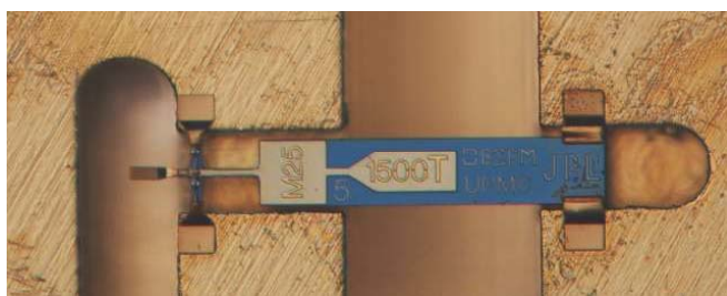
Fig.6: Photo of the 1.4 THz tripler device mounted in its waveguide block, featuring 2 anodes on 3 μm GaAs membrane in a biasless configuration.
