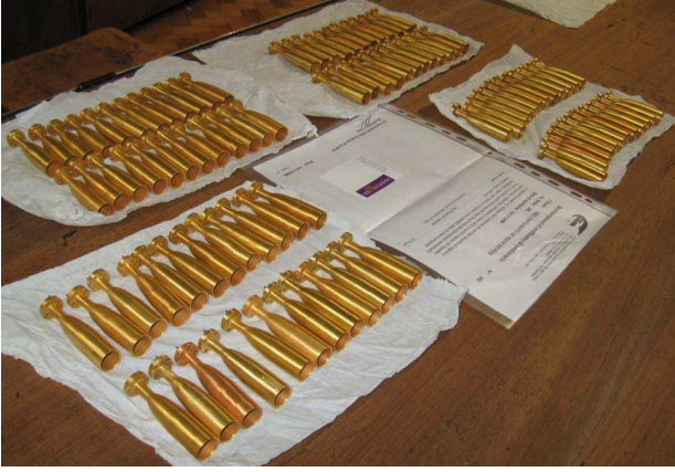
Fig. 3 The full set of 96 corrugated feedhorns for the LF focal plane.
