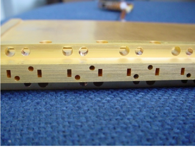
Fig. 12 Close-up view of assembled LF detector module showing split-block rectangular waveguides and circular alignment holes.
