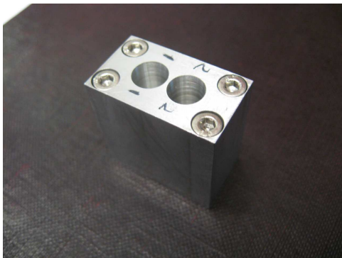
Fig. 9. The two horn array prototype, made by repeated drilling into a single block of aluminium.
