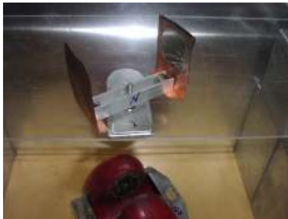
Fig. 10. Photo of rotatable aperture with Cu shield at one side and 10 dB NDF at other side. Below is the magnet by which we can precisely rotate the aperture, to place Cu shield, NDF, or OPEN between the bolometer and the window.
