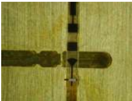
Figure 1 (a) Photograph of the 162 GHz doubler inside the split block waveguide (b) doubler efficiency plot
