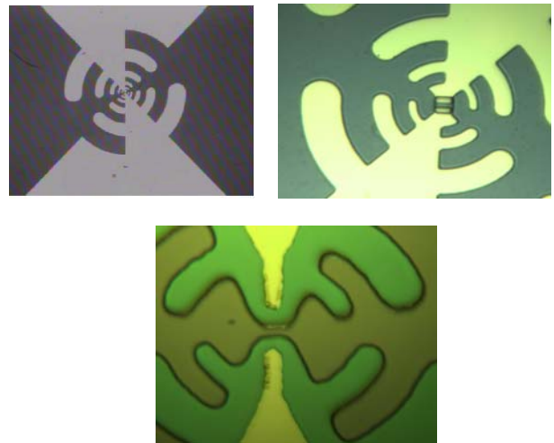
Figure 1. Different terahertz log-periodic antennas used in this work: LPA2 (top left); LPA3 (top right) and LPA4 (bottom).
