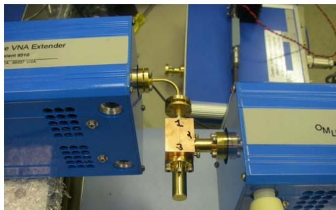
Fig. 12. Photo of the OMT during Pol 1 transmission measurement with the vector network analyser.
