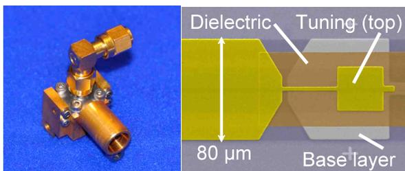
Fig. 2 *Left*: Assembled 600 GHz SMA mixer block. *Right*: SEM image of a 660 GHz SIS device fabricated at Univ. of Köln.
