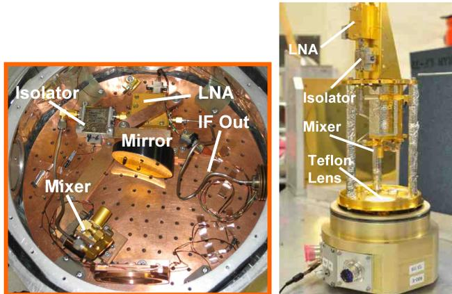
Fig. 4 *Left*: Photograph of interior of IR Labs liquid helium cryostat (4K cold plate). *Right*: Photo of upgraded 600 GHz SMA receiver insert cartridge. Vacuum window is located on the bottom along with feed-through connections. The radial o-ring vacuum seal on the cartridge is also visible.
