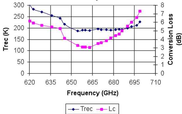
Fig. 6 Measured  $T_{\text{rec}}$  (left, blue) and mixer conversion loss (right, pink) over the 620-696 GHz frequency range for a receiver insert with an upgraded 660 GHz mixer operating in the laboratory SMA cryostat.
