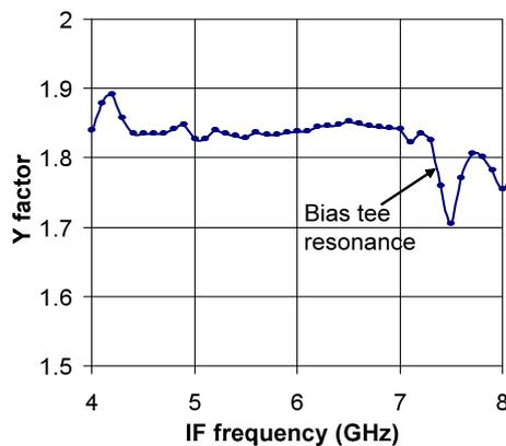
Fig. 7 Y-factor measurements made at 632 GHz over the 4-8 GHz IF passband for an upgraded 660 GHz receiver in the SMA cryostat. Measurements made from 3-9 GHz in steps of 0.1 GHz looking at a room temperature and liquid nitrogen cooled loads. Resonance effects with the bias tee used to provide SIS device bias are apparent at  $\sim 7.5$  GHz.
