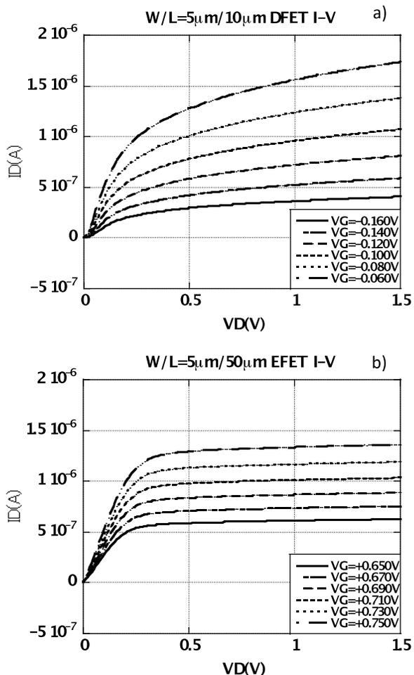
Fig. 1. Typical cryogenic (4.2 K) “ID-VDS” of the GaAs-JFETs when  $V_S=0V$ . The gate size of a) is width of  $5\ \mu m$  and length of  $10\ \mu m$ . And a) is depletion type (when  $V_G=0V$ ,  $I_D \neq 0A$ ) FET. The gate size of b) is width of  $5\ \mu m$  and length of  $50\ \mu m$ . And b) is enhancement type (when  $V_G=0V$ ,  $I_D=0A$ ) FET.
