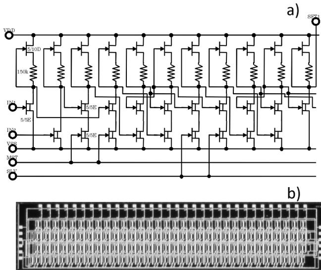
Fig. 4. The circuit diagram of the flip-flop (a) and the picture of 32-channel shift register IC (b). “5/10D” means it is depletion type JFET which gate size is width of 5  $\mu$ m and a gate length of 10  $\mu$ m. And “5/5E” means it is enhancement type JFET which gate size is width of 5  $\mu$ m and a gate length of 5  $\mu$ m.
