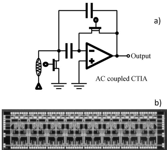
Fig. 2. The circuit concept of the AC-coupled CTIA (a) and the picture of 16-ch AC-coupled CTIA IC (b).
