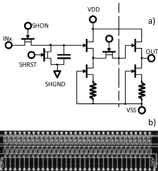
Fig. 3. A part of circuit diagram of the multiplexer with sample-and-holds (a) and the picture of 32:1 multiplexer with sample-and-holds IC (b).
