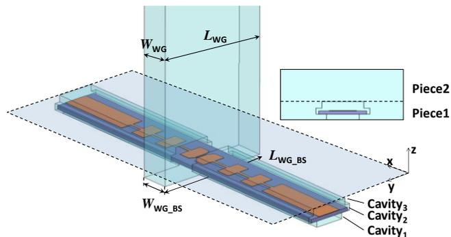
Figure 1: HEB Mixer structure designed at 1.46 THz then scaled up 2.7 THz. The plane XY materializes the mixer split-block concept which consists of a horn piece followed by the waveguide ( $L_{WG}$ ,  $W_{WG}$ ) and a back piece in which is defined a channel crossed by the waveguide backshort ( $L_{WG\_BS}$ ,  $W_{WG\_BS}$ ). The chip is inserted into the channel.
