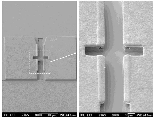
Figure 2: Electron microscope image of the channel structure consisted of stack of 3 gold layers of 5, 4 and  $5 \mu\text{m}$ -thick, respectively and realized by means of the UV-photolithography and the micro-plating technique.
