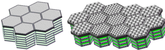
Fig. 11. CAD drawing of the proposed POLARBEAR-2 focal plane (left) and LiteBIRD focal plane (right). POLARBEAR-2 focal plane mounts seven heagonal wafers with lumped diplexer with total of 7588 bolometers. LiteBIRD focal plane uses two types of detectors. There will be eight low frequency wafers with larger lenses and five high frequency wafers near the center of the focal plane. LiteBIRD focal plane will have 2022 bolometers total.
