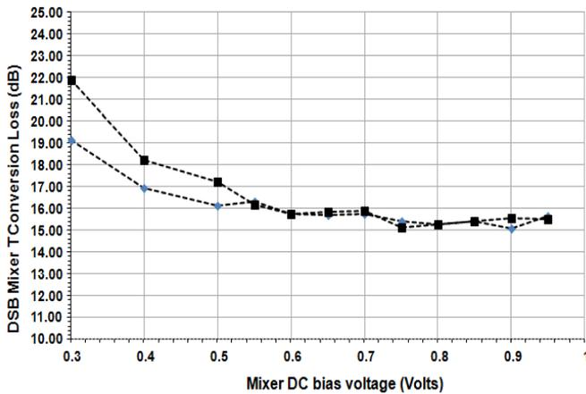
Fig.3. Preliminary measurement results of the 1200 GHz sub-harmonic mixer VS DC bias voltage of both diodes in series. Top: DSB mixer noise temperature. Bottom: DSB mixer conversion losses for two blocks under test. Available LO input power: 1-1.5 mW. Center frequency: 1193 GHz.
