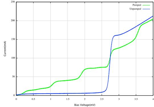
Fig. 8. The IV and IF characteristic of the SIS mixer tested with LO injection at 208.8 GHz.
