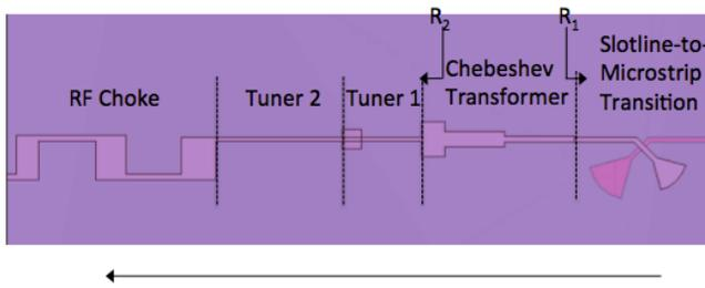
Fig. 2. Magnified view of the broadband power coupling and tuning network around the SIS junction, consisting of a Slotline-to-Microstrip Transition, a Chebyshev Transformer, Tuner1, Tuner2 and an RF Choke. The arrow indicates the power propagation direction.
