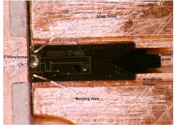
Fig. 3. The SIS mixer chip mounted in the WR4 waveguide, supported by grooves on either side of the waveguide. The SIS mixer is connected to the IF transformer by 25  $\mu\text{m}$  diameter aluminium wires. The mixer block provides a ground connection to the device via bonding wires at either sides of the device.
