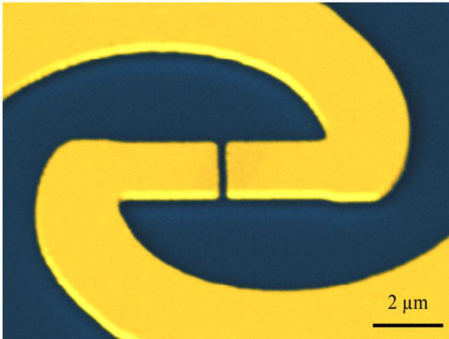
Fig. 2. SEM image (colorized and tilted view) showing the inner part of a log-spiral antenna and the gap between electrodes where the HEB is located.
