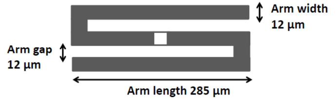
Fig 2: Folded dipole antenna structure with number of turns N=3 .
