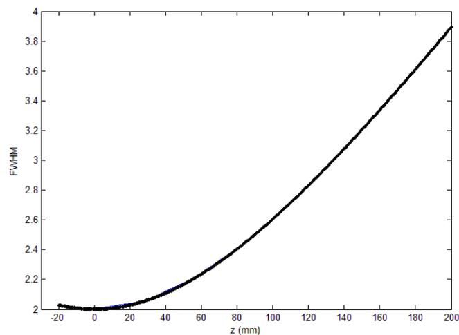
Fig. 3. Beam waist distribution in function of Z. The curve refers to the LW band array.
