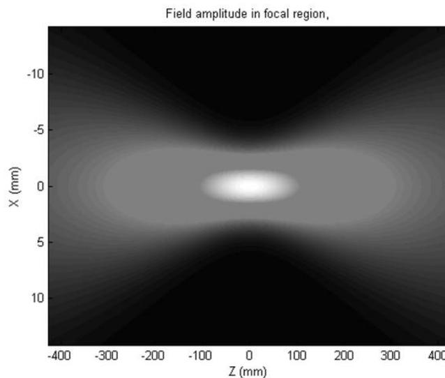
Fig. 2. Field amplitude in the focal region. The field in function of Z is calculated using a Gaussian beam approach.
