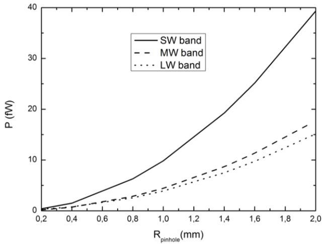
Fig. 6. Optical loading on the TES bolometers for the 3 bands in function of the pinhole sizes.
