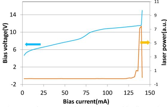
Fig. 4. Measured current vs voltage (I-V) curve (blue line) and current vs laser power characteristics (red line) at heat sink temperature of 15K. The maximum laser power is  $\sim 100\mu\text{W}$  in CW mode.
