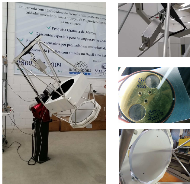
Fig. 5 – Left: the complete HATS system assembly undergoing operational tests. Right, top: the Golay cell and double window wheel front-end case at the Newtonian focus; middle: chopper wheel with 0.87 and 1.4 THz band-pass filter windows; bottom: the 46 cm rough surface reflector with three small polished mirrors for alignment adjustments.
