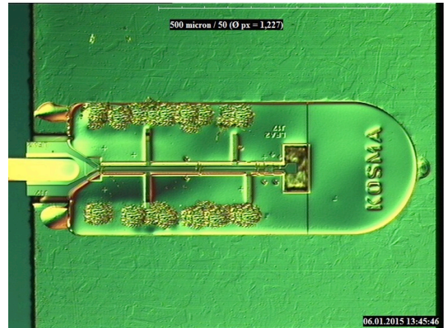
Fig. 2 Microscope photograph of a LFA HEB device mounted on its waveguide block. The use of difference interference contrast shows subtle height differences and explains the false colour of the gold layers.
