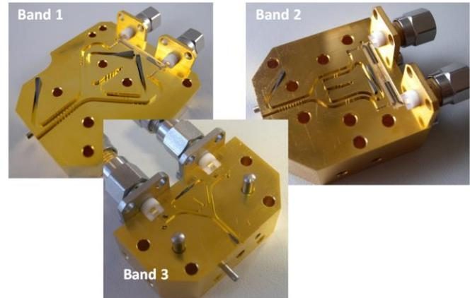
Fig. 3 Sideband separating SIS mixers for NOEMA Band 1, 2 and 3.
