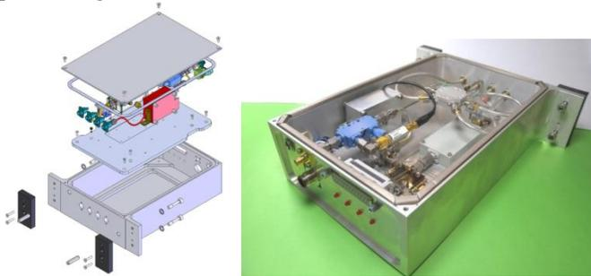
Fig. 5 Warm IF amplification module with integrated switch and digital attenuator.
