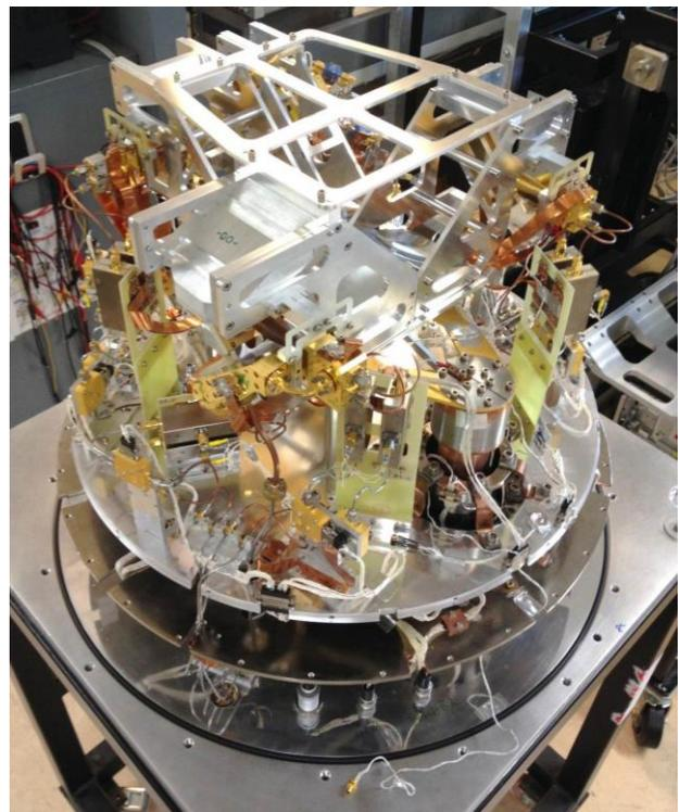
Fig. 8 View of the cold sections of the NOEMA Front-End.
