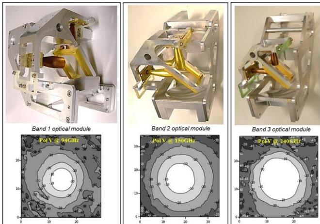
Fig. 2 Cryogenic optics modules for NOEMA Bands 1, 2 and 3 (top panels) and Pol V copolar beam patterns measured with the antenna range near the central frequency of the respective RF ranges (bottom panels).
