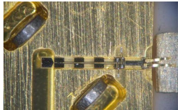
Fig. 4. Sideband Separating Mixer developed for NOEMA Band 3 (200-276 GHz) showing details of one of the two DSB mixer chips of the 2SB assembly with miniature magnets to suppress the Josephson effect.
