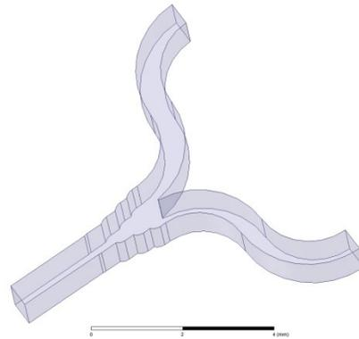
Fig. 4 Design of -3dB E-plane power splitters.
