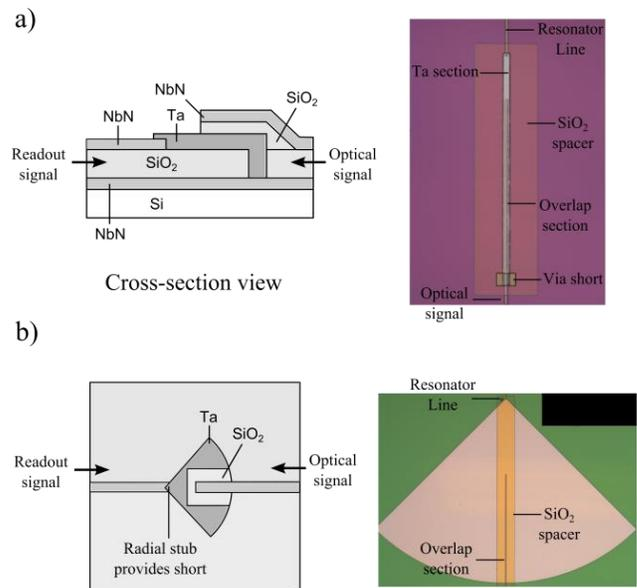
Fig. 4 Optical coupling schemes. a) Overlap design b) Radial stub design.
