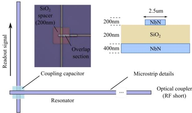
Fig. 5 Details of resonator microstrip.
