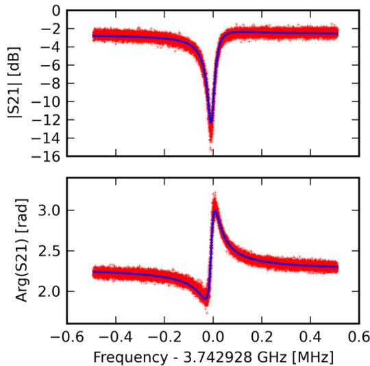
Fig. 6 Measured resonance curve for a via-shortened test resonator. Upper plot shows the transmission gain measured and the lower plot the transmission phase shift, as measured with a VNA. The fitted values for the unloaded and coupling Q-factors are  $1.98 \times 10^5$  and  $8.3 \times 10^4$  respectively. The readout power is estimated to be approximately -107dBm at the device. This is a preliminary measurement made without the optimised readout system, hence the relatively high noise level.
