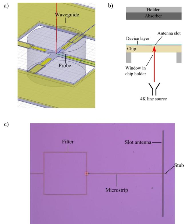
Fig. 2 Details of antennas for CAMELS chips. a) Proposed 4-probe horn coupling. b) Concept for test devices. c) Photo of realised antenna on test device.
