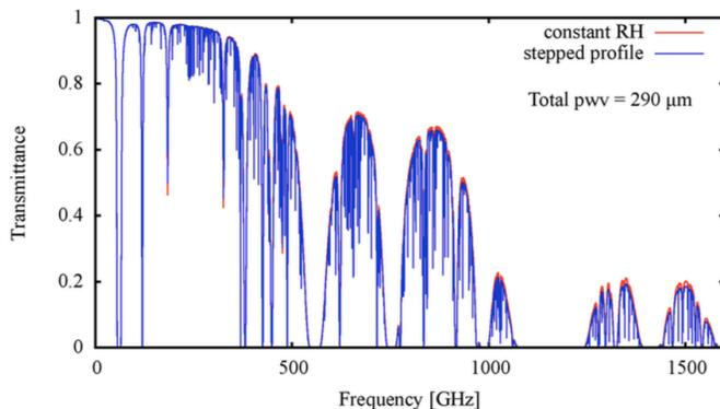
Fig. 1. Predicted atmospheric transmittance for the ALMA site under dry conditions [2].
