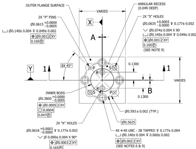
Fig. 3. Schematic of the VDI High Precision waveguide interface for use at WM-164.
