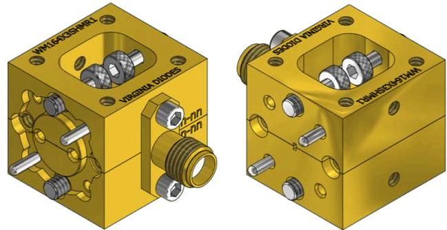
Fig. 4. Two views of the WM-164X3SHM, which consists of a broadband tripler followed by a full-band subharmonic mixer. The left view shows the WM-164 high precision waveguide interface, and the right view shows the input waveguide at WR-4.5.
