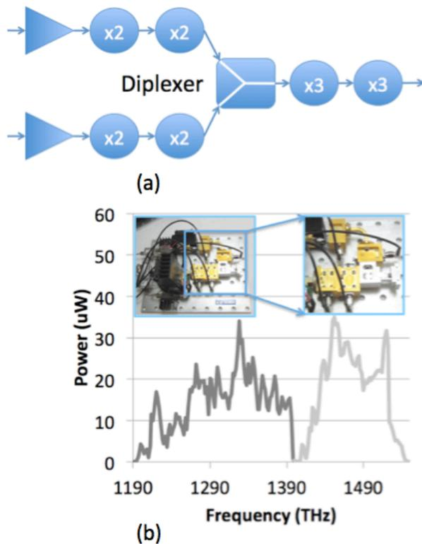
Fig. 5. (a) Basic architecture of 1.25-1.51 THz Source and (b) measured output power from a previous prototype of the source, showing the two varactor chains combined using the waveguide diplexer.
