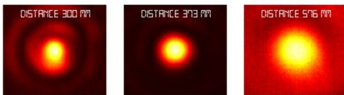
Fig. 2: Beam profiles of the LO at 300, 373, and 576 mm distance from the TPX lens (from left to right). The profiles were measured with a microbolometer camera. The width of each snapshot is 4.5 mm and the height 4 mm.
