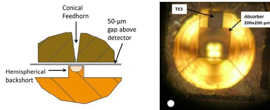
Figure 1. Left: Cross-section of feedhorn and hemispherical backshort showing position of detector. The diameter of the hemispherical backshort is 500  $\mu\text{m}$ . Right: Photograph of detector sitting above hemispherical backshort. The absorber is a thin Ta film with a sheet resistance close to 377 ohm. The white circle in the lower left-hand corner indicates the size of the feedhorn's exit aperture.
