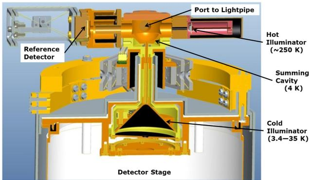
Figure 2 overview of the calibration source and the summing cavity. The black cone is a variable temperature calibration load. At the apex of the cone is a 400 μm pinhole (not visible at this scale) that is connected to the summing cavity via light pipe.
