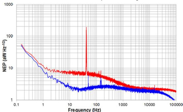
Figure 3 NEP values of the TES detector with the light pipe closed (blue) and open (red). The increase in NEP with the light pipe open is
