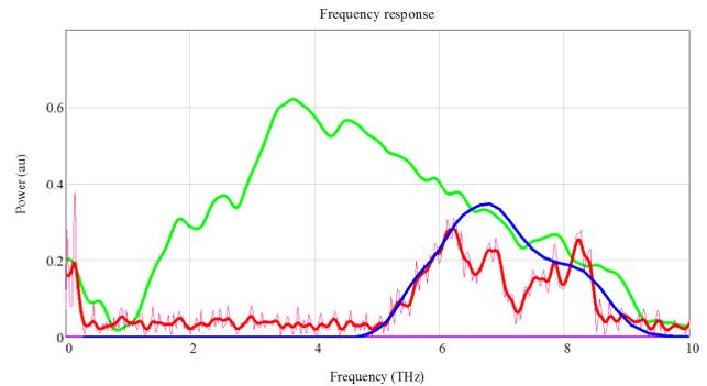
Figure 5 Measured spectrum of the reference detector (green) and the SW-pixel (red). The blue curve is the transmission of the SW filter stack (measured separately)
