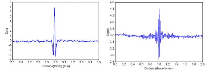
Figure 4 Left: (part of the) interferogram of the reference detector. Right: interferogram of the SW TES detector
