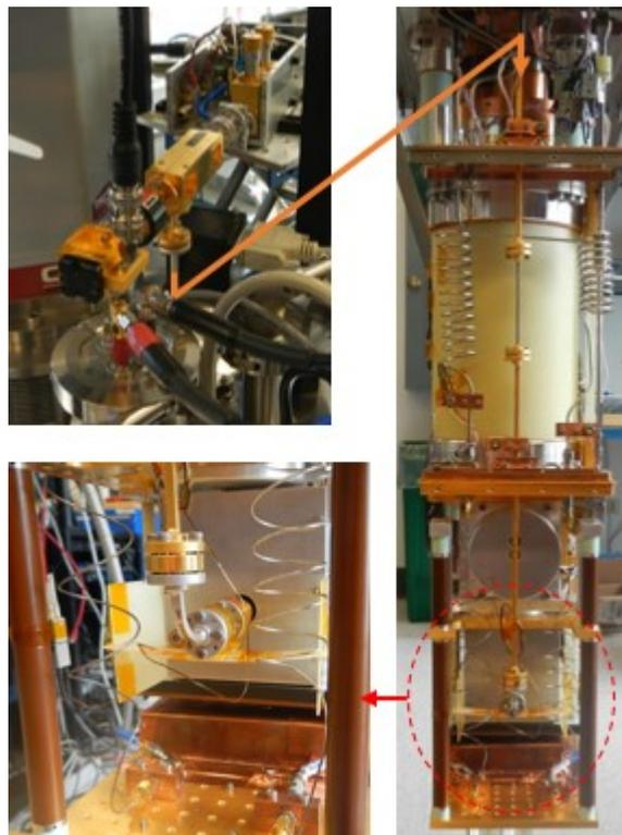
Fig. 3 Upper left: the millimeter wavelength source, coupler, isolator, and diode detector. Right: waveguide plumbing. Lower left: detailed view of the horn and entrance to the optics box.
