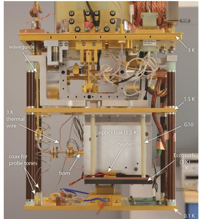
Fig. 1 Detailed photograph of the test setup. The device under test is attached to the 100 mK plate at the bottom of the image. In the configuration shown, the copper thermalizing plate is above the Eccosorb slab. When the external millimeter wavelength source is used, the copper plate is below the Eccosorb so that reflections in the optics box are terminated in the absorber.
