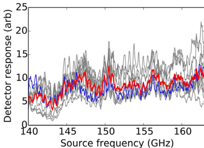
Fig. 4 Example spectral response measurement of an array of aluminum LEKIDs obtained using this setup. Each of the gray curves shows the response of a single detector. The response of a single detector is highlighted in blue for clarity. The average response across the array is shown by the thick red curve. The fringing is due to reflections in the test setup rather than the intrinsic detector response, and can be corrected for.
