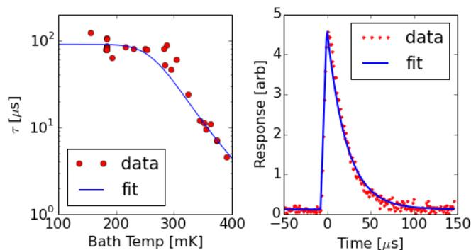
Fig. 5 Left: example time constant data from an aluminum LEKID, measured as a function of bath temperature. The time constant saturates below 300 mK because of background illumination from the Eccosorb. Right: The device response to a 2  $\mu$ s wide pulse of radiation from the millimeter wavelength source.
