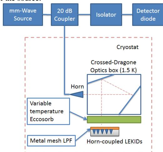
Fig. 2 Simplified schematic of the test configuration.
