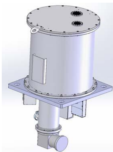
Fig. 2. View of the dual-band receiver showing the signal and calibration windows, and placement of the cryogenic cold-head and control electronics. Warm optics is not shown.
