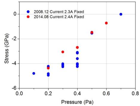
Fig. 3 The dependence of film stress on sputtering pressure.
