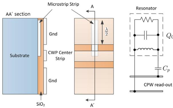
Fig. 1 The layout configuration (not in scale) and the circuit diagram of the test sample.
