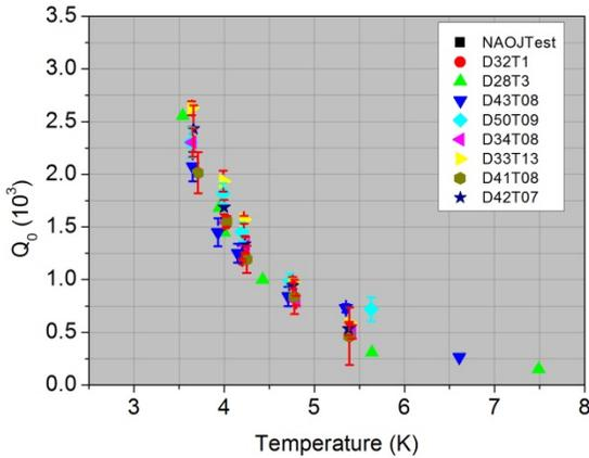
Fig. 5 The dependence of  $Q_0$  on ambient temperature of samples. These samples have different resistivity but show similar  $Q_0$ .
