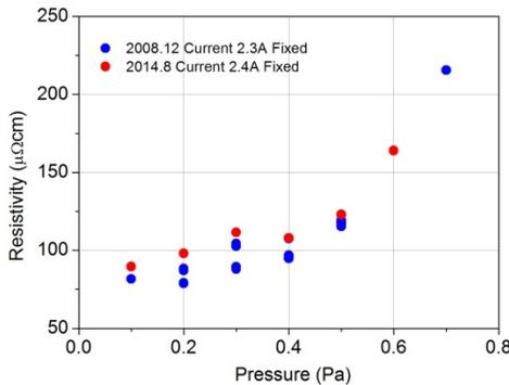
Fig. 2 The dependence of film resistivity on sputtering pressure.
