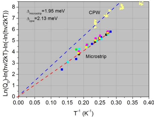
Fig. 7. Extraction of energy gap according to Mattis-Bardeen theory
