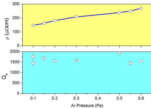
Fig. 6 The  $Q_0$  measured at 4K and the resistivity of NbTiN as a function of sputtering pressure.
