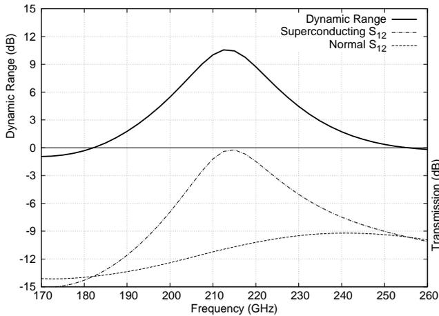
Fig. 6. The response of a superconducting on/off switch with two 50 nm thick NbN nano-bridges separated by a quarter wavelength long slotline.
