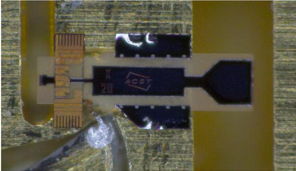
Fig. 3 Device mounted in the split-block, ready for testing
