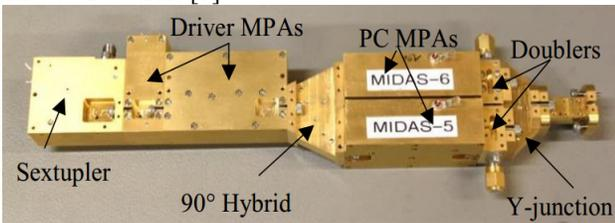
Fig. 4 Power combined amplifier/doublers for the high power 200GHz test source (courtesy of Bertrand Thomas, RPG GmbH)
