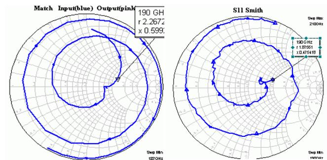
Fig. 11 S11 (input of tripler) simulated (left) and measured (right)
