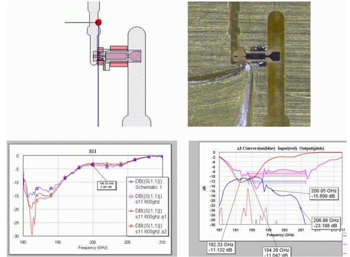
Fig. 10 machining error discovered, and updated simulation including error
