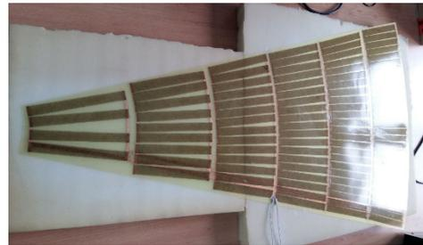
Fig. 8 Pattern of the de-icing film heaters.
