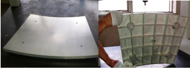
Fig. 1 Prototype aluminium panels for DATE5
