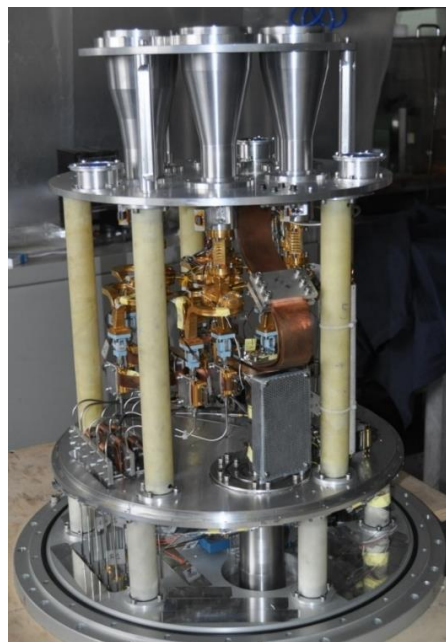
Fig. 4. Photo of the K-band seven-beam front-end showing the assembly of the components inside the cryostat (external shields removed).
