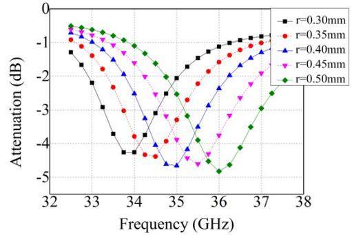
Figure 3. Attenuation vary with the probe radius
