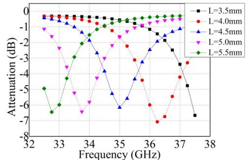
Figure 5. Attenuation vary with the coaxial length
